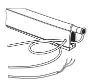
Slide the emitter and receiver into the upper chamber. Guide the emitter cable through the lower chamber to the receiver side.
